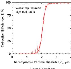
Figure 3. VersaTrap performance at 15L/min.
