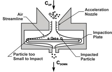
Figure 1. Schematic of an inertial impactor
